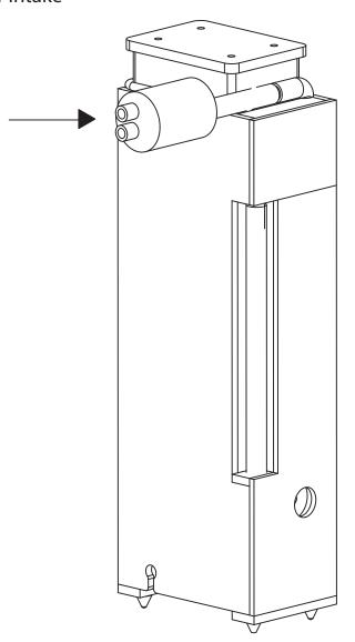
When placing your skimmer in the skimmer column, make sure the air intake is facing towards the rear of the aquarium.
