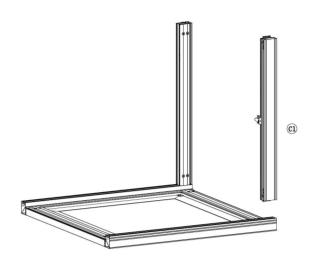
2.) Attach Top or Bottom Rear Profile (C) to (A & B) and lock into place. Make sure the profiles line up with the end caps.
