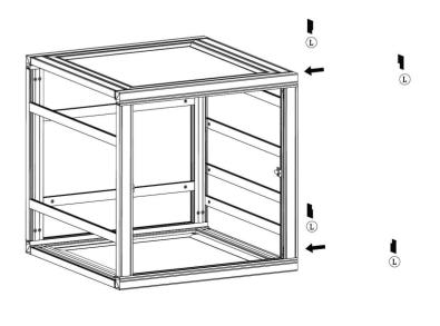
11.) Flip stand onto its base and make sure all profiles are locked and stand is level.
