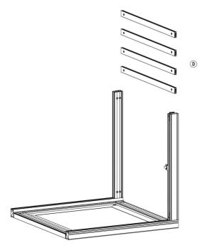
5.) Attach Top Profile (C) to the top of (A & B) and lock into place.
