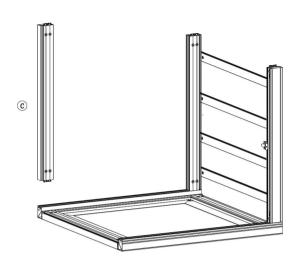
6.) Attach Top Front Profile (C2) to the top of (A & B) and lock into place.
