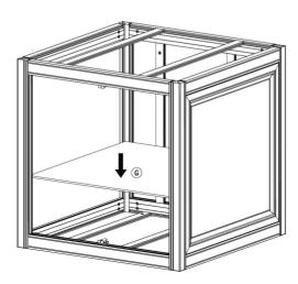
13.) Insert the door (M) into the white pivot brackets. Slide the door to the left and tighten top and bottom pivot brackets using a phillips head screwdriver.
