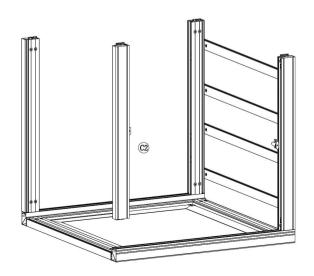
7.) Attach Horizontal Cross Profiles (2  $\times$  D) between (C and C2) and lock into place.
