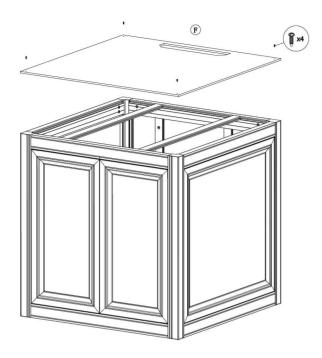
16.) Using a box cutter, cut and remove the pre-scored hole on panel (F)
