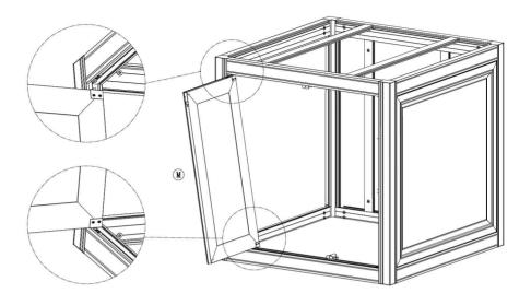
14.) Repeat step 16 with door (M1). Slide the door to the right and tighten top and bottom pivot brackets using a phillips head screwdriver.
