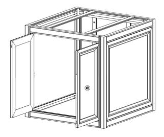
15.) Screw panel (F) into the end caps with the provided  $4 \times 10^{-5}$  x phillips head screws.
