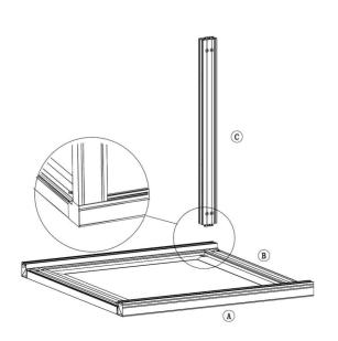
4.) Attach Horizontal Cross Profiles (4 x D) to (A & B) and lock into place.
