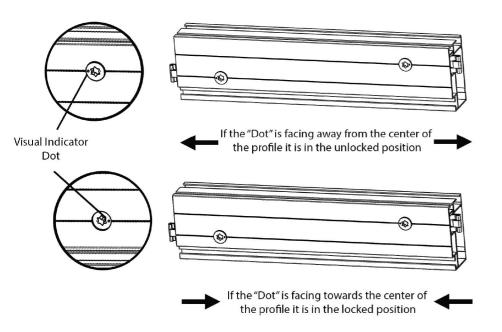
When assembling the stand the profile's tension locks utilize the smaller channel.
