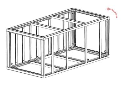
7.) If stand is not level, loosen and move profiles to readjust.
