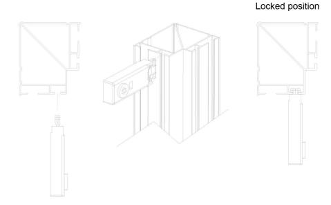
To securely lock each profile into position, insert the supplied hex torque wrench into the tension lock and turn clockwise.
