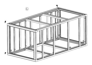
6.) Flip stand onto its base and make sure all profiles are locked and stand is level.
