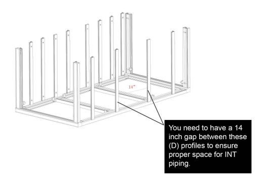
4.) Attach Rear Profile Frame (B) to frame and lock into place.
