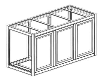
8.) Insert bottom board (G) and screw panel (F) into the end caps with the provided 4 x phillips head screws.
