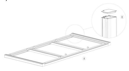
2.) Attach Top and Bottom Side Door Profiles (C1 & C2) to (A) and lock into place. Make sure the profiles line up with the end caps.
